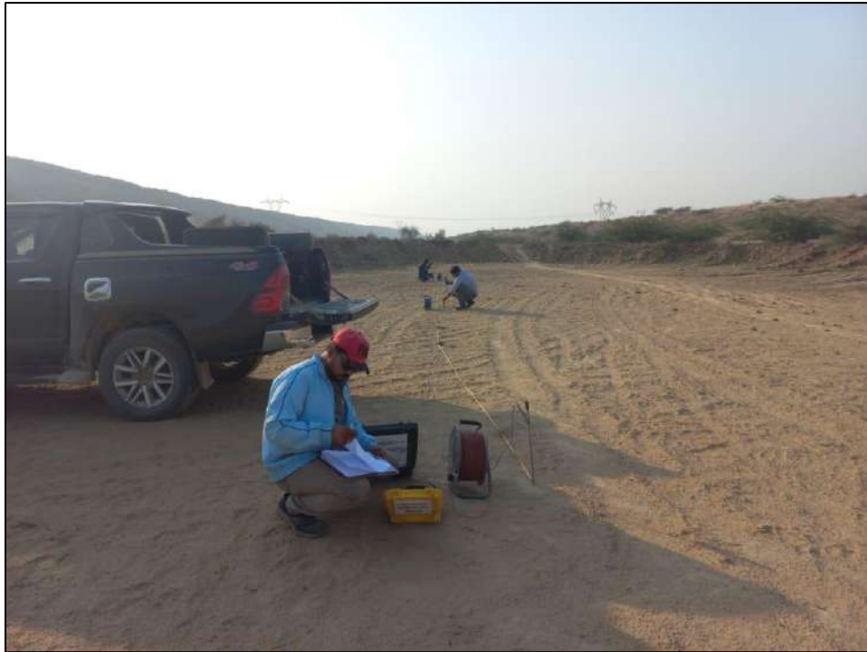
Figure 4.2 Electrical resistivity Test in progress
