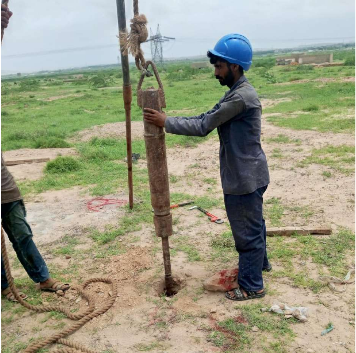
Figure 3: Standard Penetration Test in progress
