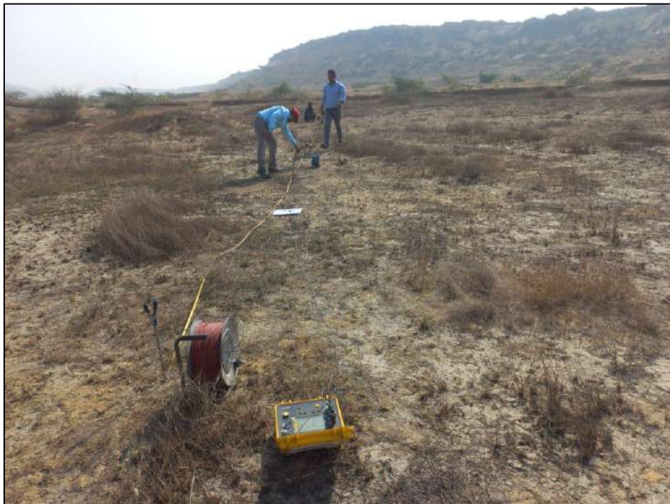
Figure 4.3 Electrical resistivity Test in progress
